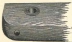
End of Evener Showing Malleable Bushing
